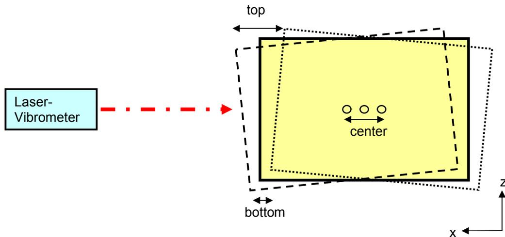
Figure 3. Illustration indicating how a rocking motion of big objects affects the measurement of linear movement.
