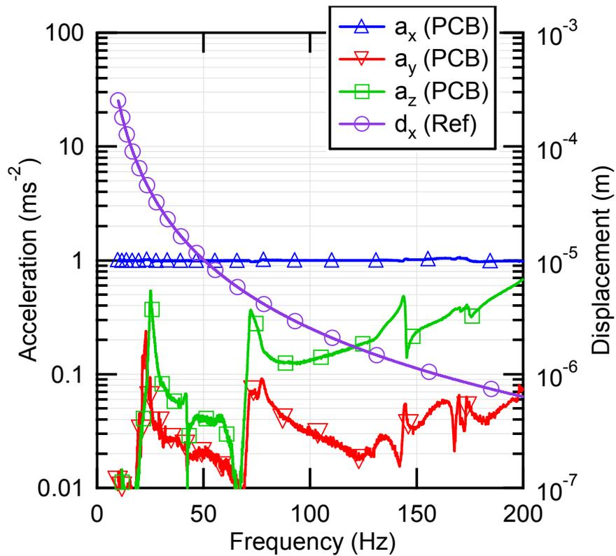
Figure 5 Table movement of the optimized mounting configuration: the three acceleration components were measured by a small triaxial
