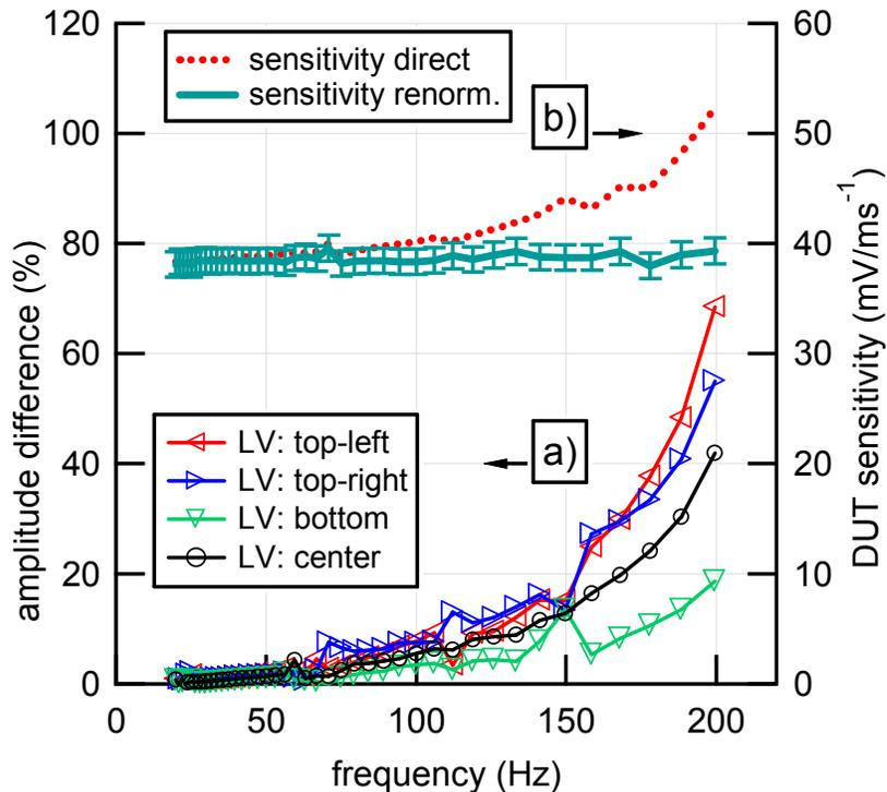
Figure 6. Calibration of the DUT using an additional laser vibrometer, performed with the shaker at METAS:
