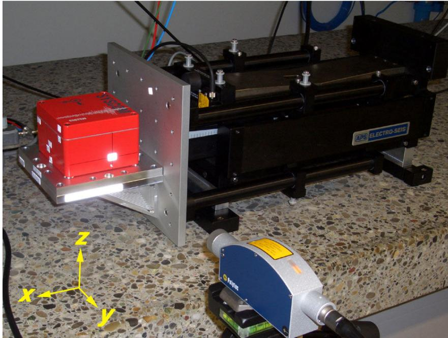
Figure 4. Optimized mounting configuration for which the resulting driving force vector acts onto the center of mass of the total moving structure.
