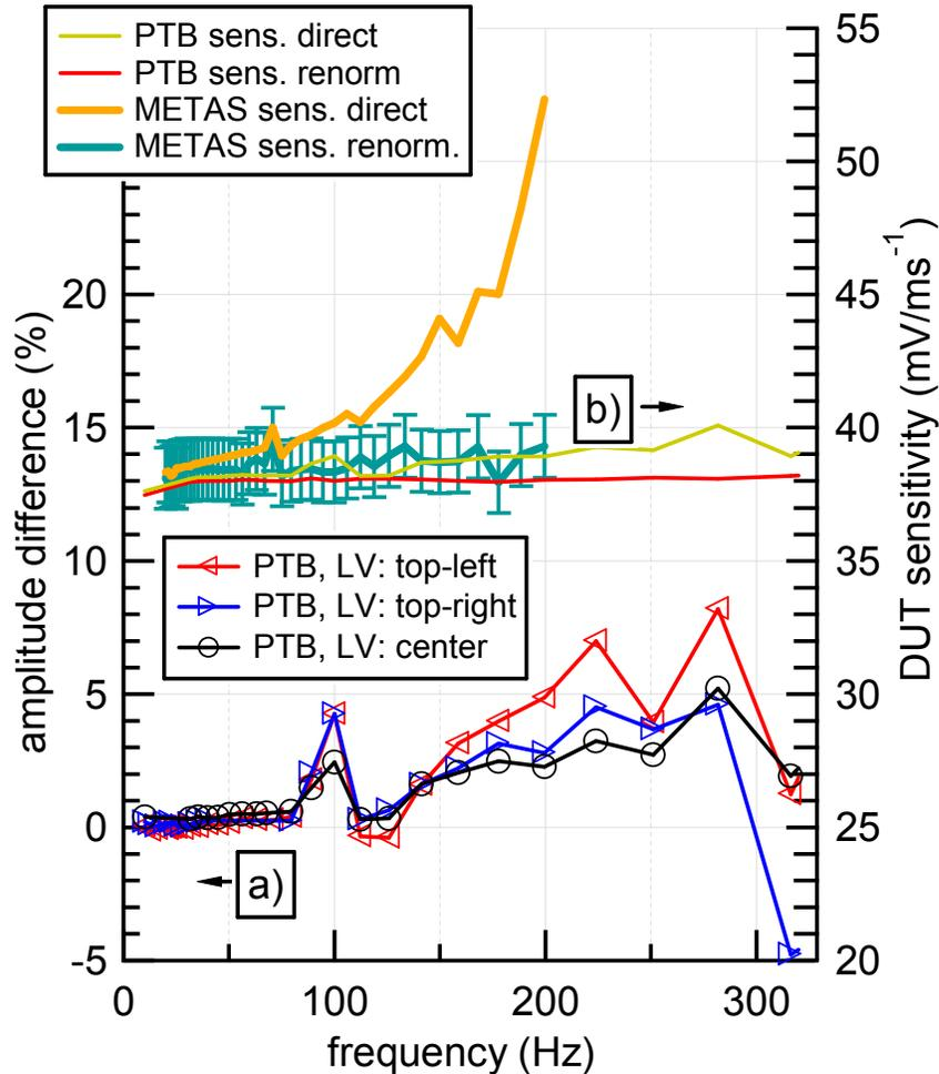
Figure 8. Calibration of the DUT using an additional laser vibrometer, performed with the multi-component shaker at PTB:
