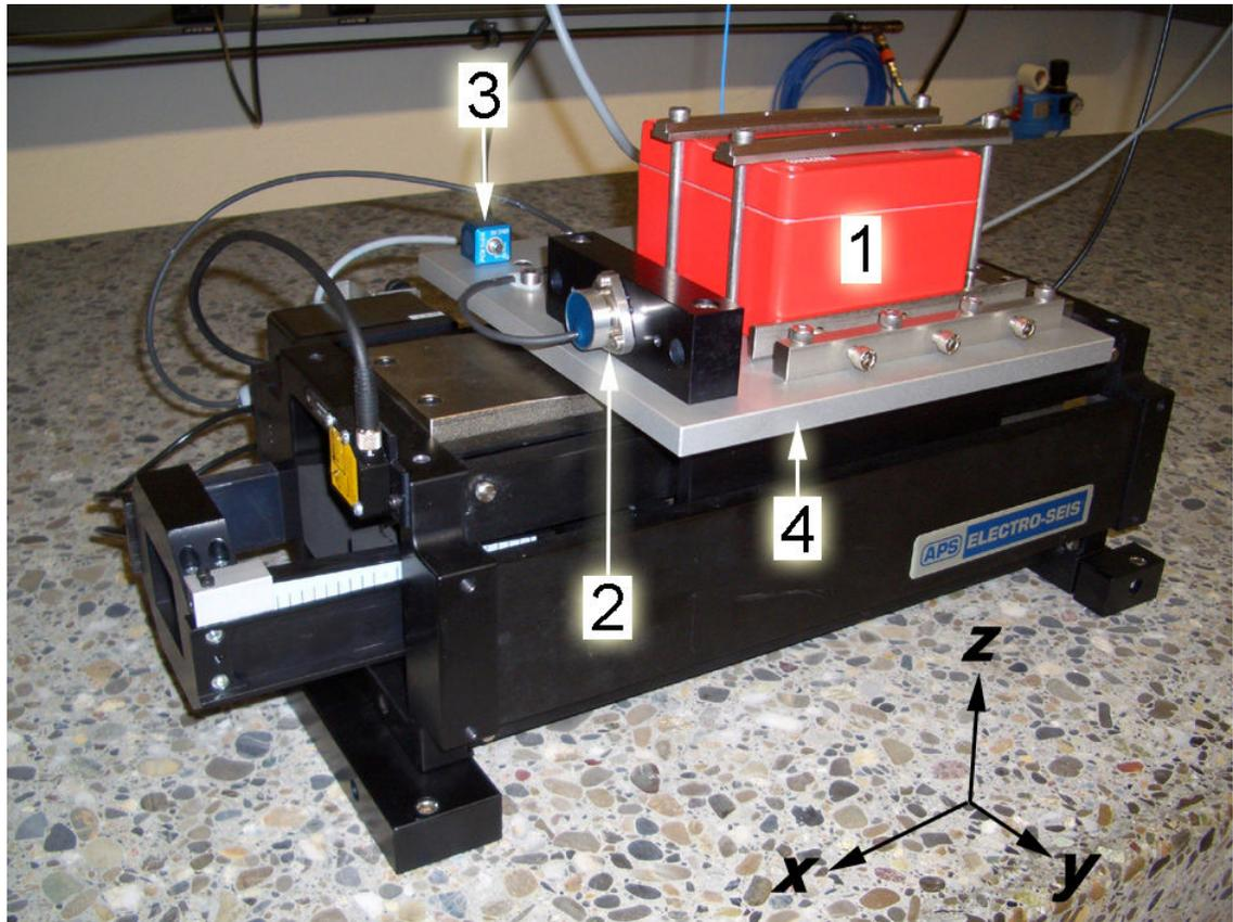
Figure 1. Original mounting configuration of the DUT (1), reference sensor (2) and monitoring triax (3) on the auxiliary table (4) of the APS-113 shaker in horizontal operating mode
