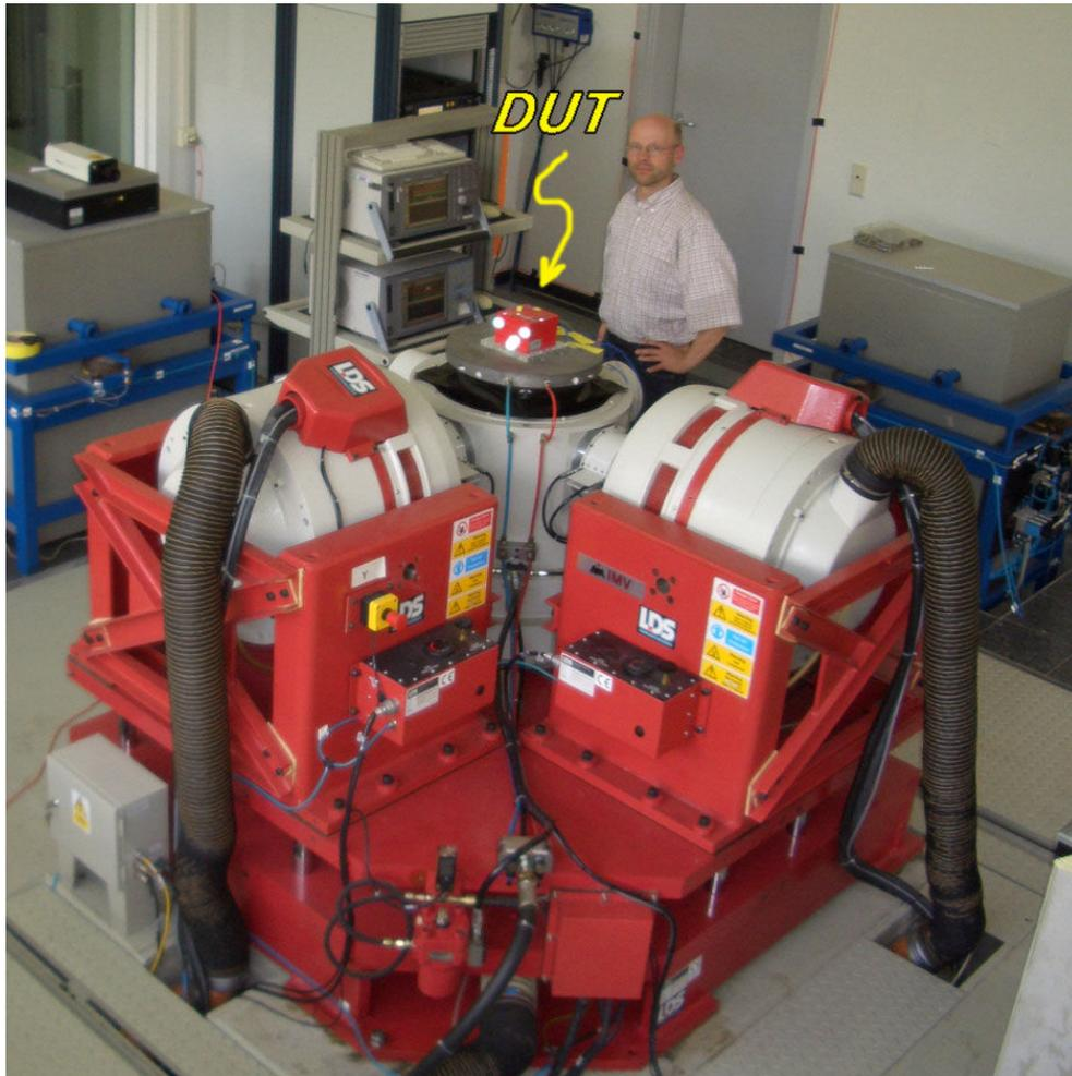
Figure 7. View of the multi-component exciter available at PTB. This shaker provides mechanical excitations of outstanding quality. Rocking motion is suppressed to large degree.
