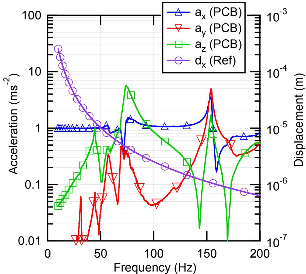
Figure 2. Table movement of the original mounting configuration: the three acceleration components were measured by a small triaxial accelerometer (PCB), the nominal displacement was obtained from a reference accelerometer (Ref).
