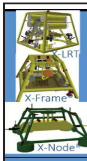
*Fig. 2. The bottom unit in Fig.1 includes an X-node (docking stations) with permanent cable connection and an instrumented exchangeable top unit (X-Frame) that can be launched and recovered with the Launch-Recovery Tool (X-LRT) developed by partner (Metas AS). The ARIM X-frame includes the iCrawler garage (see Fig. 1). This allow user to operate and maintain the ARIM system without the assistance of expensive vessel time.*
