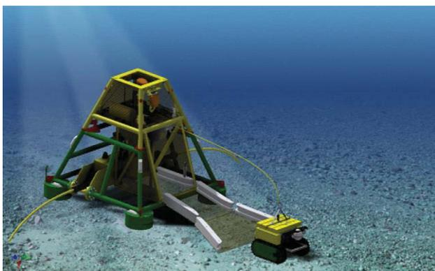
*Fig. 1. The ARIM benthic platform with mobile crawler equipped with cameras and oceanographic sensors. The garage platform supports charging of batteries while the connecting cable enable communication between crawler and garage during training of crawler autonomous operations.*
