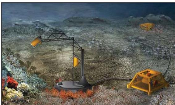
*Fig. 3. The LoVe observatory with stationary acoustic and imaging sensors. The camera to the left images routinely a coral reef while the vertical and horizontal acoustic sensor mounted on the platform to the right monitor the full water column. Illustration Equinor ASA.*
