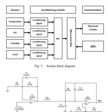
Fig. 4. pH probe circuit sensing
