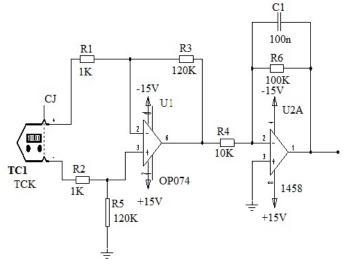
Fig. 6. Temperature interfacing circuit
