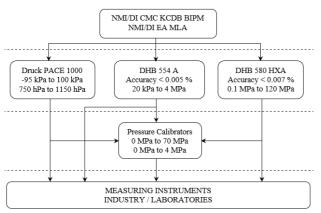
Figure 3: Traceability scheme for the Laboratory for Pressure
