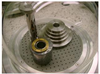
Figure 2. Piston and Weights of the Pressure Balance.
