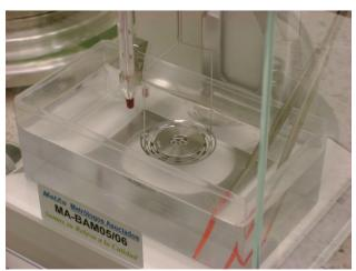
Figure 3. Density Determination by Hydrostatic Comparison of a Weight (10 g).
