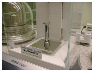
Figure 5. Mass Calibration of a Piston (almost 100 g).
