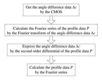
Fig. 4: Algorithm chart of the measurement
