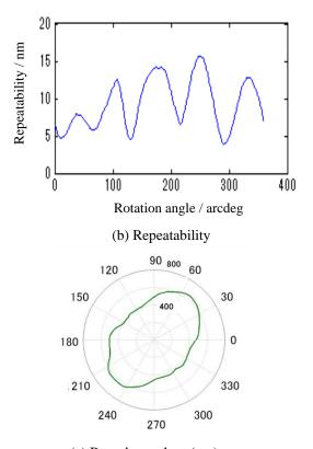
(c) Roundness chart (nm) Fig. 6: Profile, repeatability and roundness figure of cylinder measured by MBAS
