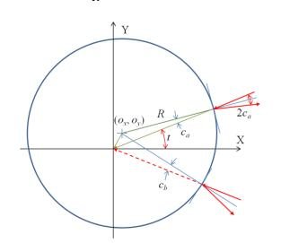
Fig. 3: Relation between eccentricity and reflected beam:  $o_x$ ,  $o_y$ : center of cylinder (eccentricity), *R*: radius of cylinder,  $c_a$ ,  $c_b$ : measured angles by MBAS, *t*: converging angle
