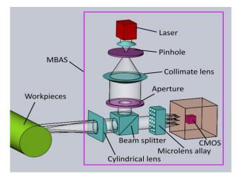
Fig. 1: Construction of the Multi-Beam Angle Sensor
