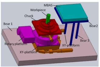
Fig. 2: Schematic of MBAS system
