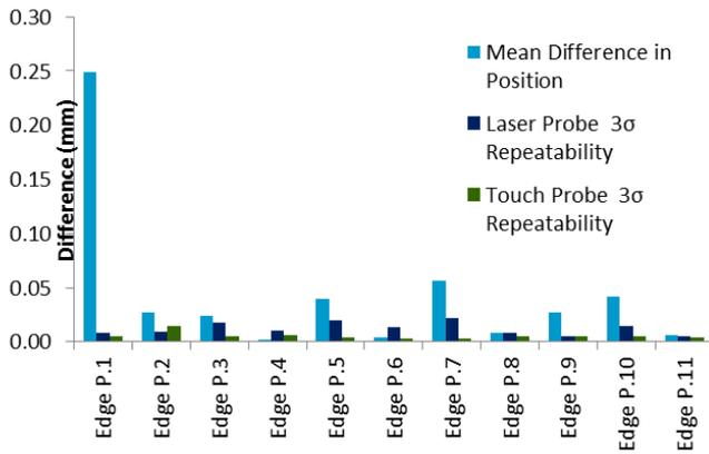
Fig (6): Edge points measurement results in 3σ repeatability distribution.
