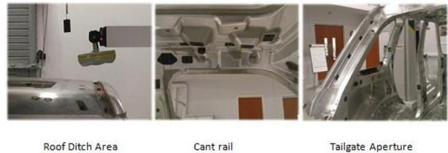
Fig (4): Examples of some features which cannot be evaluated by XC65Dx laser line scanner.
