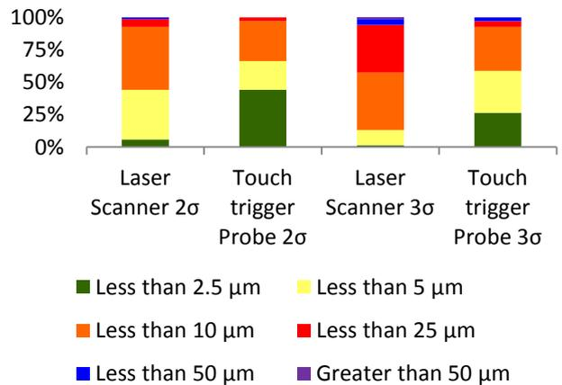
Fig (5): Points measurement results in  $2\sigma$  and  $3\sigma$  repeatability distribution.
