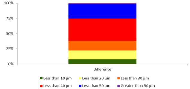
Fig (7): Difference between laser scanner and touch trigger probe measurement values.
