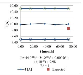
Figure 1: The calibration history and expected value in a single point of current measurement range
