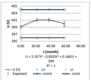
Figure 2: The calibration history and expected value in a single point of voltage measurement range
