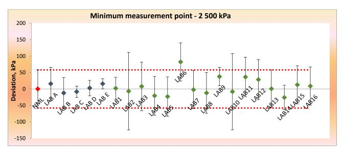
Figure 3: Participant's deviation from the reference value and its corresponding uncertainties at 2 500 kPa
