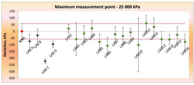
Figure 4: Participant's deviation from the reference value and its corresponding uncertainties at 25 000 kPa
