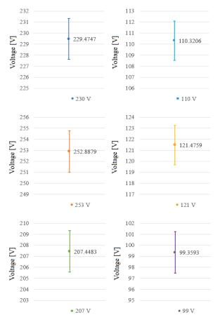
Figure 3: Graphical representation of the expanded uncertainty of the PQ generator – RMS voltage
