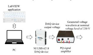
Figure 1: A schematic representation of the virtual PQ disturbance generator and its components
