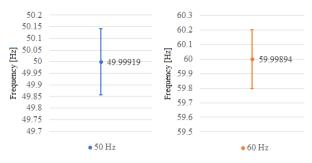
Figure 4: Graphical representation of the expanded uncertainty of the PQ generator – frequency
