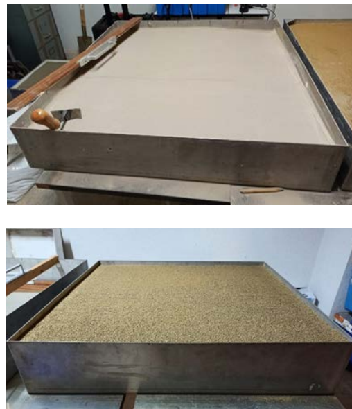
Figure 2: Picture of the Exhalation Beds: Brown, to the top: high radon flux, grey, to the bottom: low radon flux.
