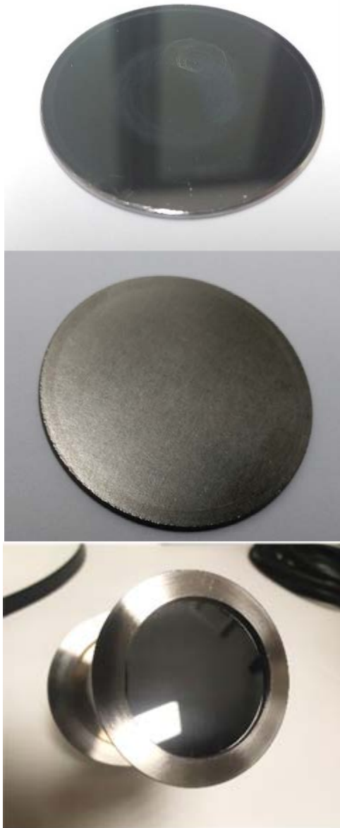
Figure 1: New kind of activity sources for ^{222}\text{Rn} based on the principle of emanation from electro-deposition, implantation or vapor layered ^{226}\text{Ra} activity standard. From top to bottom: Electro-deposited ^{226}\text{Ra} activity standard: Deposition at 30 \text{ V} < U < 200 \text{ V} ; Implanted ^{226}\text{Ra} activity standard: Implantation of ^{226}\text{Ra} into W / Al after mass separation; PIPS ^{226}\text{Ra} activity standard: 450 \text{ mm}^2 , 300 \mu\text{m} with 150 \text{ Bq} ^{226}\text{Ra} layer.
