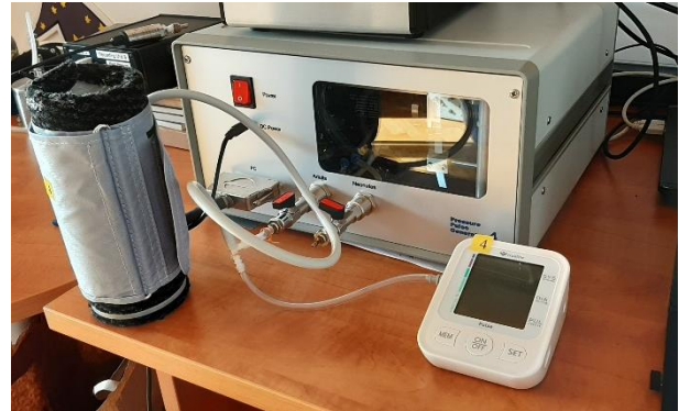
Figure 3: Example of test setup, sphygmomanometer connected to the aOSG.
