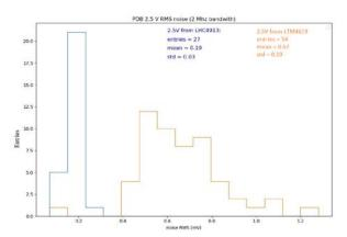
Figure 5: Histogram of noise RMS of LTMs and LHCs 2.5 V outputs
