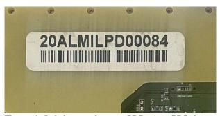
Figure 4: Label example on a PDB. Any PDB has a barcode that is a unique code.
