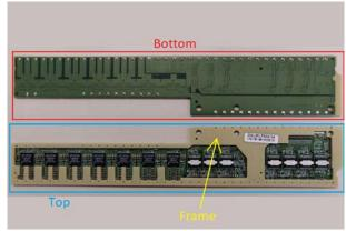
Figure 2: Picture of a PDB as seen from the top and the bottom. All components are mounted on the top side. On the same side, the G10 reinforcement frame is also visible. Picture from [3]
