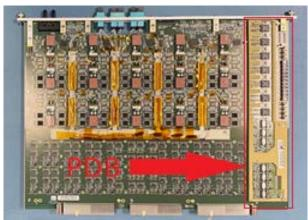
Figure 3: Picture of the PDB mounted on the LTDB. The PDB is located on the right side of the picture. Picture from [3]
