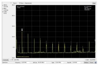
Figure 7: Noise spectrum of LHC4619 with 2.5 output voltage
