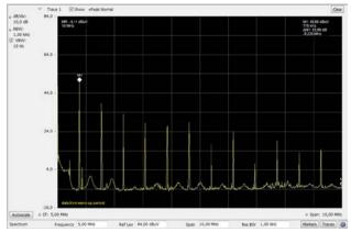
Figure 6: Noise spectrum of LTM4913 with 2.5 output voltage
