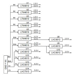
Figure 1: Power scheme of the PDB. The board integrates LTM4619 DC/DC converters (U1-U7) and LHCx913 linear voltage regulators (U8-U14) to produce the voltages needed by the LTDB (the number of devices has been established based on the budget of the output currents). From the two +6 V lines available on the input power bus, one (labelled "6 V") is used to generate the digital voltages and the other one "6 VA" is used to generate the analog voltages. Picture from [3]
