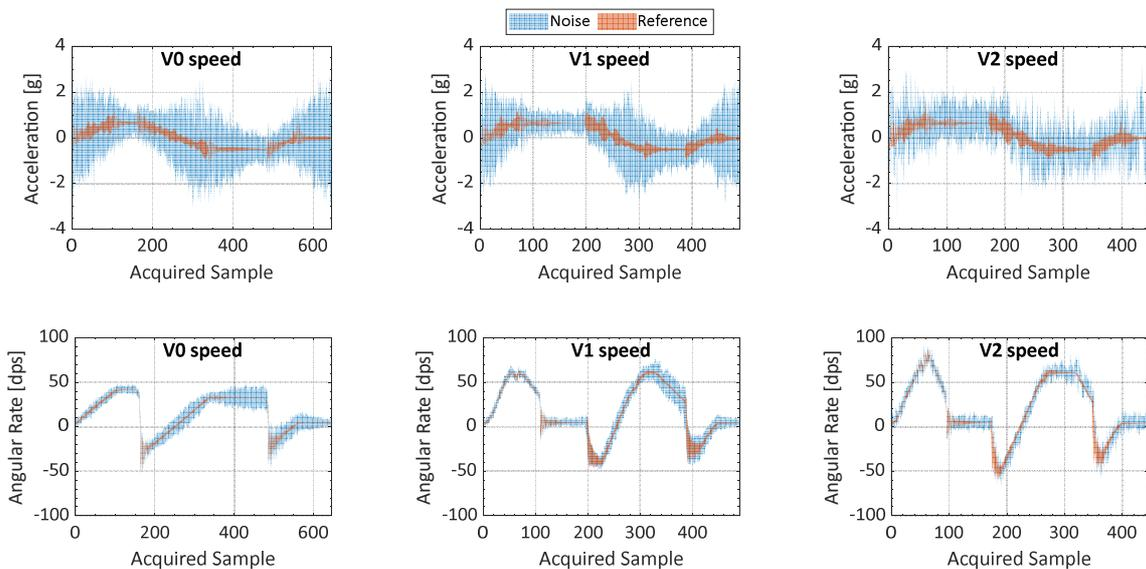
Fig. 2. Comparison between signal acquired in presence of noise (blue area) and without noise (red area). Top subplots refer to accelerometer with different speed sets, bottom subplots refer to gyroscope with different speed sets.
