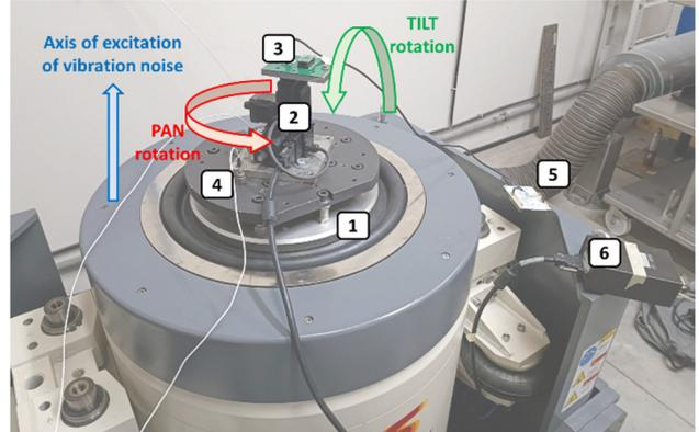
Fig. 1. Picture of the entire experimental setup for dynamic characterization of IMU: 1) shaker, 2) PTU; 3) MEMS-based IMU under test; 4) control accelerometer; 5) acquisition board; 6) PTU controller.
