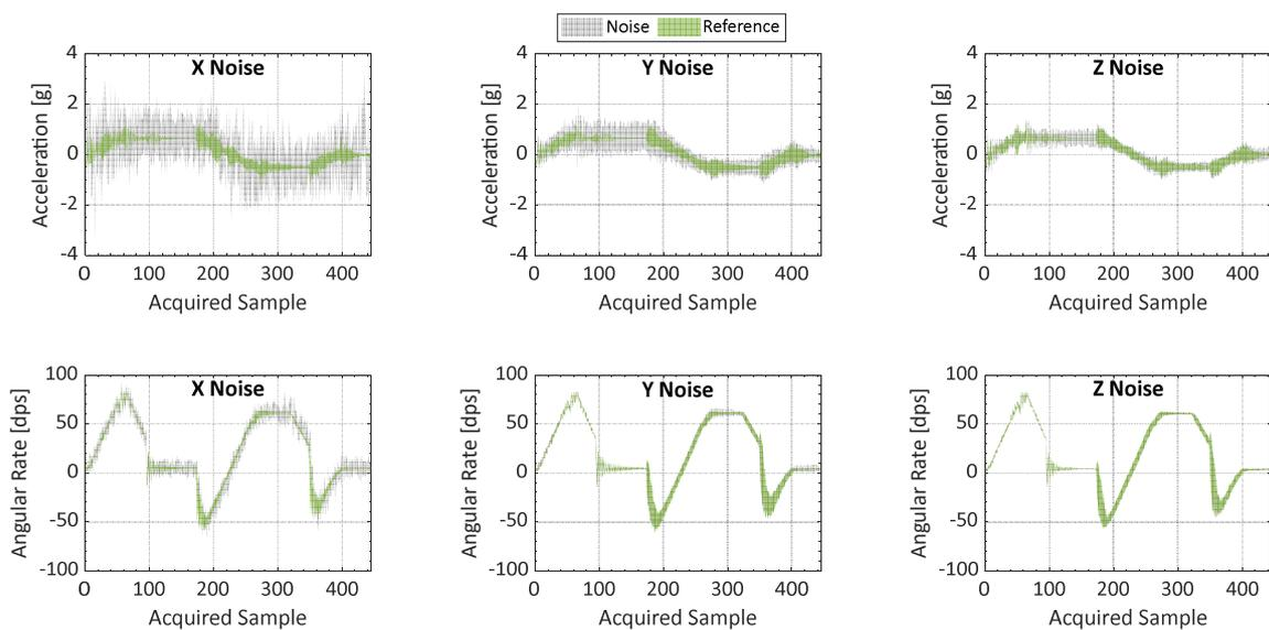
Fig. 3. Comparison between signal acquired in presence of noise (grey area) and without noise (green area), considering noise applied toward different directions.
