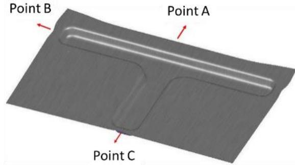
Fig. 2. T-joint geometry with points where the draw-in is measured
