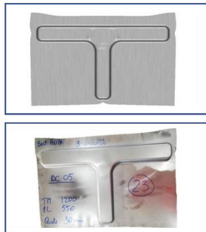
Fig. 4. Numerical-experimental comparison profile of the drawn component under optimal condition.
