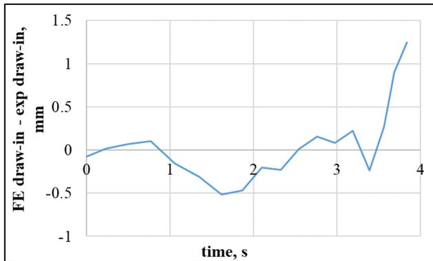
Fig. 5. Numerical and experimental comparison in the draw-in of one blank.
