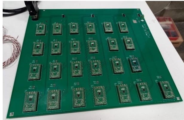
Fig. 1. Picture of the devices under test mounted on a customized board.
