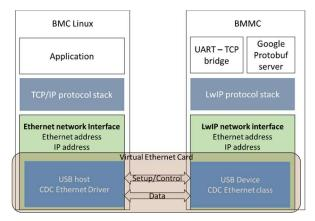
Fig. 6. CDC Ethernet communication between the BMC and BMMC
