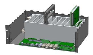
Fig. 1. A plan of an 8 slot BRAINE Edge Micro Data Center [2]
