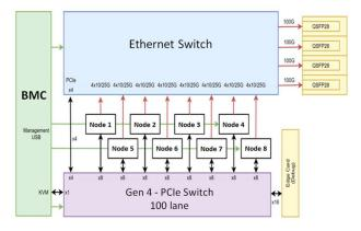
Fig. 2. Architecture of the BRAINE Edge Micro Data Center [2]
