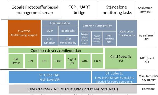
*Fig. 5. Software architecture of the Board Management Microcontroller*
