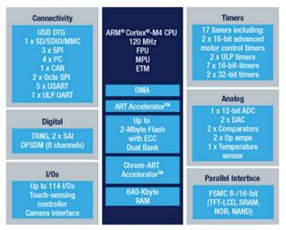
Fig. 3. Internal architecture of the Board Management Microcontroller [3]
