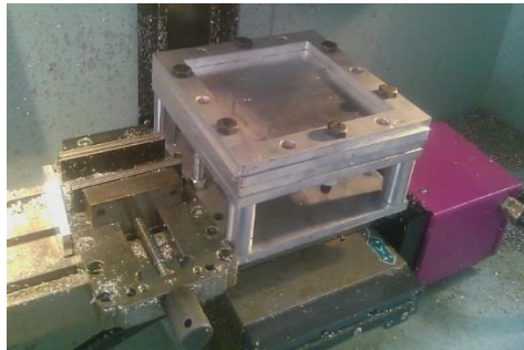
Fig. 2. Fixture and rig on the CNC machine table
