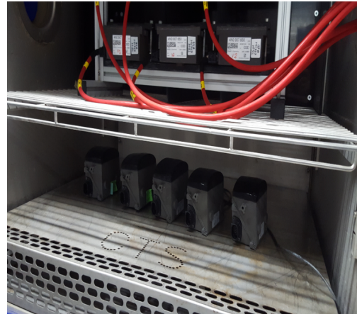
Figure 13 Product placed in climate chamber
