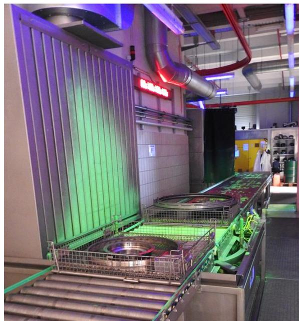
Fig. 7: Penetrant test processing line
