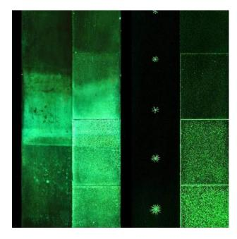
Fig. 8: »Test Panel Type 2« (left: coating corroded / right: origin condition)
