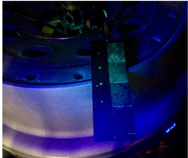
Fig. 6: Aircraft wheel rim including »Test Panel Type 2«
