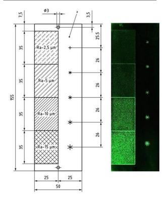
Fig. 1: »Test Panel Type 2« according to ISO 3452-3 (dimensions in mm according to ISO 3452-3 [left] and using a fluorescent penetrant [right])
