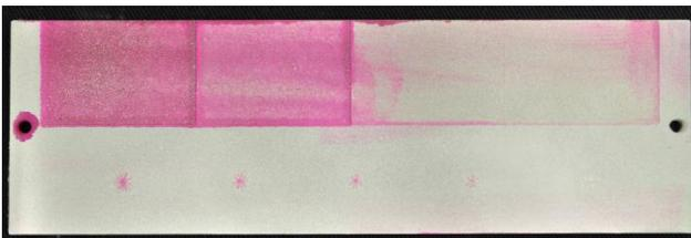
Fig. 5: »Test panel type 2« (with colour contrast penetrant)
