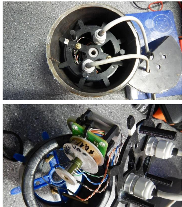
Fig. 3. The fully equipped laboratory ME sensor intended for the experiment on the patent wire P7, the assembled sensor inside the steel shield (above) and view on its disassembled basic parts (below)
