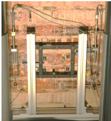
Fig. 11. Instrumentation of a masonry specimen with reference and monitoring targets for optical measurement
