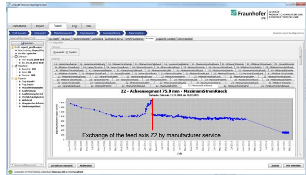
Fig. 1. Development of a feature for monitoring feed drives over a period of approx. 2 years
