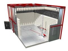
1. Fig. Semi Anechoic 3m EMC Chamber with traditional square design [3]
