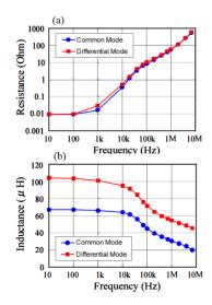
3. Fig. Calculated (a) resistance and (b) inductance of stator windings per phase for common mode and differential mode. [5]
