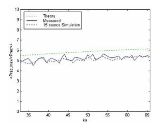
6. Fig. The estimated (theory), measured, and simulated ratio for an example EUT [1]
