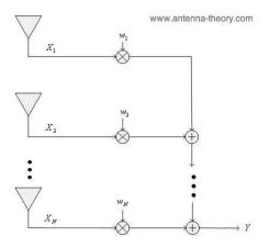
7. Fig. Weighting and summing of signals from the antennas to form the output in a Phased Array [10]
