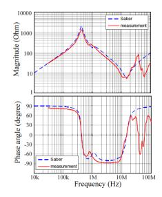
5. Fig. Frequency characteristic of motor impedance for differetial mode (magnitude and phase angle) by the equivalent circuit [5]
