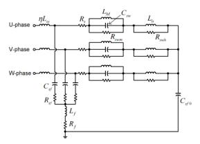
4. Fig. Equivalent circuit of a three-phase Y-connected BLDC motor. [6]
