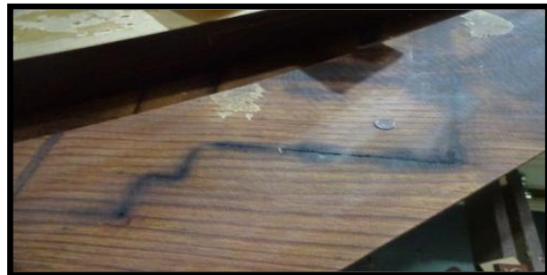
Fig-6: Formation of creep path due to continuous
