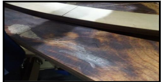
Fig-5: Burn marks on other side of the permawood ring.
