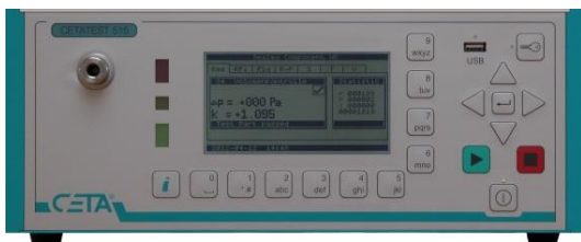
Fig. 6. Leak tester type CETATEST 515 for the leak test of encapsulated test parts with small volume [8].
