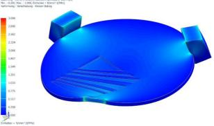
Figure 6: Von Mises stresses of the clamped disk under load. Note: third gripper finger not show in this post-processing picture and displacement five times enhanced for illustration.
