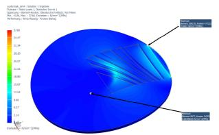
Figure 7: Von Mises stresses of the bended disk under application loads. Note: the provisions of the virtual test-rig are not shown and the displacement is five time enhanced for illustration.
