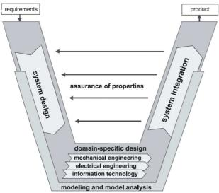
Figure 1: The V-Model according to guideline VDI 2206 [1]
