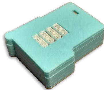
Fig. 3. 3D printed enclosure with the mounted board.
