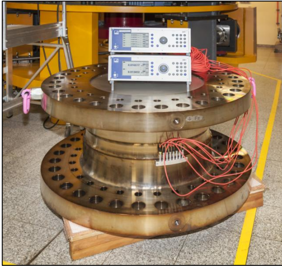
Fig. 3. 5 MN·m torque transducer together with two DMP41 bridge amplifiers for the readout of the 8 channels of the transducer.
