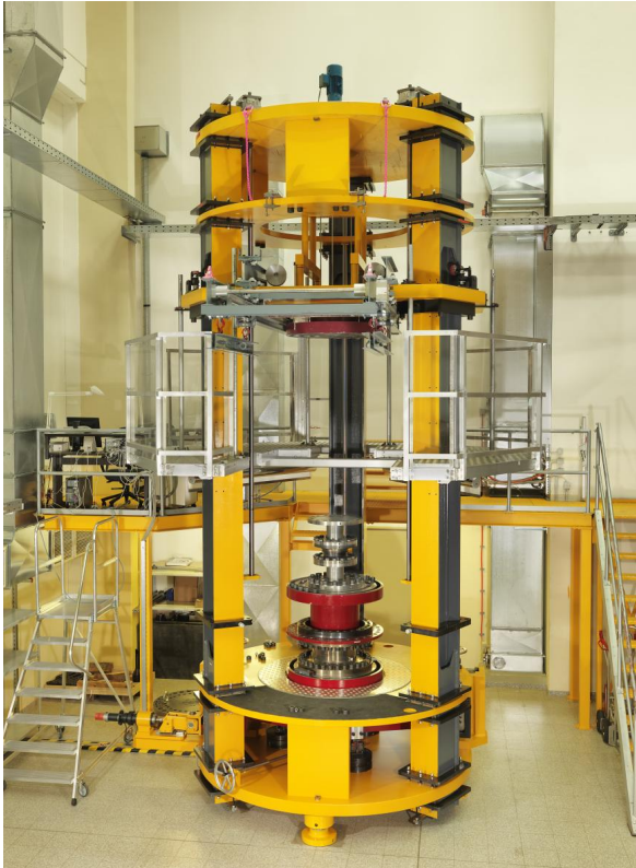
Fig. 2. The 1.1 MNm Standard Calibration Machine of PTB.
