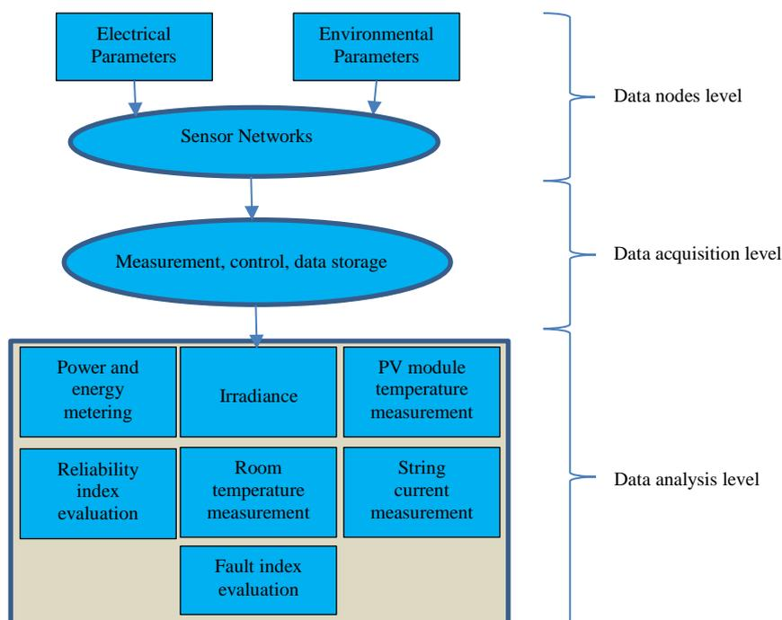
Fig. 2. PV smart monitoring system
