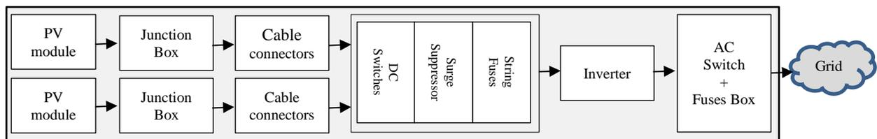
Fig. 1: Schematic diagram of photovoltaic plant.
