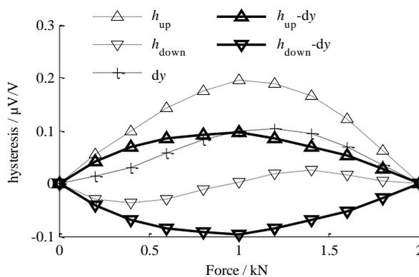
Fig. 2. Graphical representation of the hysteresis deviation  $dh$  obtained by the difference of upward  $h_{up}$  and downward  $h_{down}$  hysteresis, subtracted from the linearity deviation  $dy$ .
