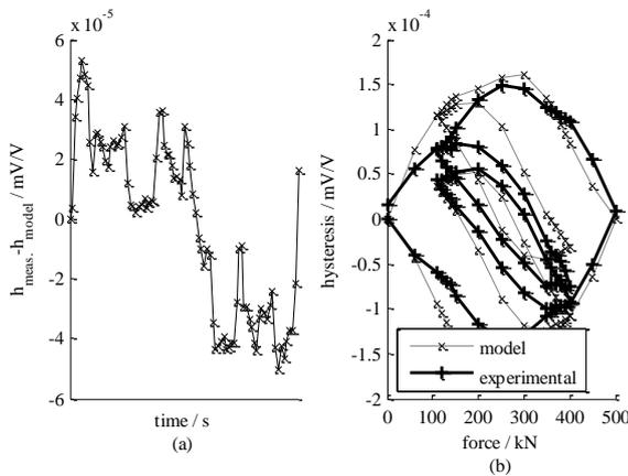
Fig. 8. Comparison between the hysteresis computed with Maxwell-Slip model and the experimental hysteresis using the transducer HBM C3H3.
