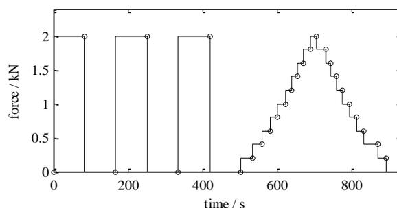
Fig. 1. Procedure for hysteresis evaluation; circles represent the measurements points.
