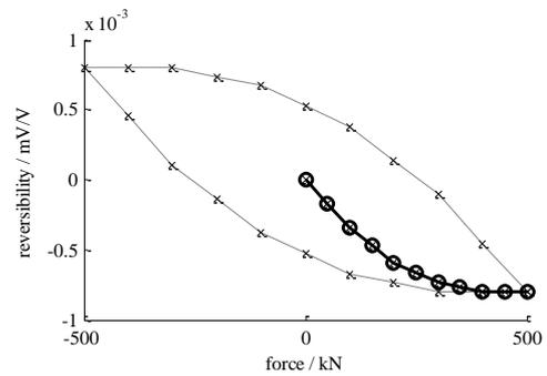
Fig. 7. Response of the force transducer HBM type C3H3, 500 kN.
