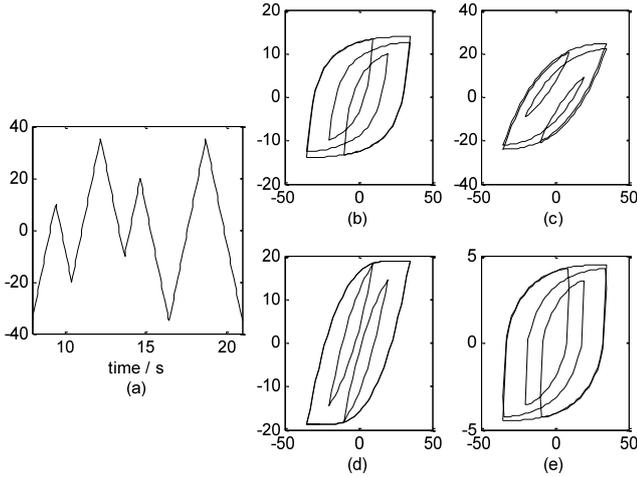
Fig. 5. Comparison of hysteresis models: (b) Dahl model, (c) LuGre model, (d) Maxwell-Slip model and (e) Bouc-Wen model, from the input temporal signal (a).
