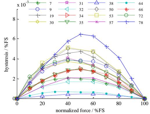
Fig. 3. Comparison of hysteresis deviation for 20 measurements made by several NMI, and for different force ranges between 1 kN up to 1000 kN.
