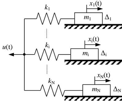
Fig. 6. Maxwell-slip model.
