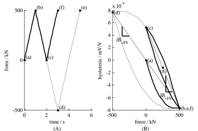
Fig. 4. Test procedure with small hysteresis loops depend on time (A) and displacement (B)
