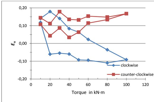
Fig 11:  $E_n$  comparison of a calibration ( DIN 51309 ) with the data by PTB
