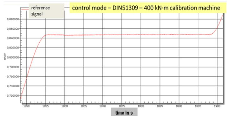
Fig.9: Signal in mV/V during a measuring step (30 s)
