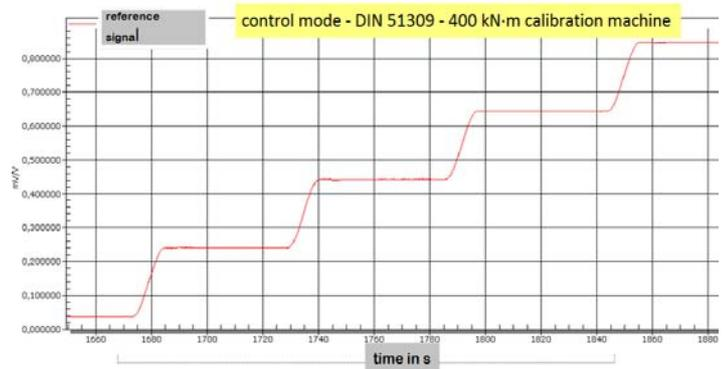
Fig.8: Clockwise load steps in mV/V according to DIN 51309
