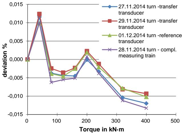
Fig 10: Comparison between the 400 kN·m reference transducer calibration (ccw) at HBM and PTB (01.04.2014)
