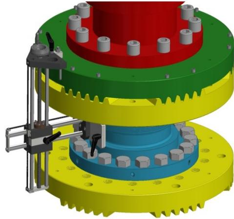
Fig.4. The test specimen (blue) mounted between the toothed adapters (yellow)
