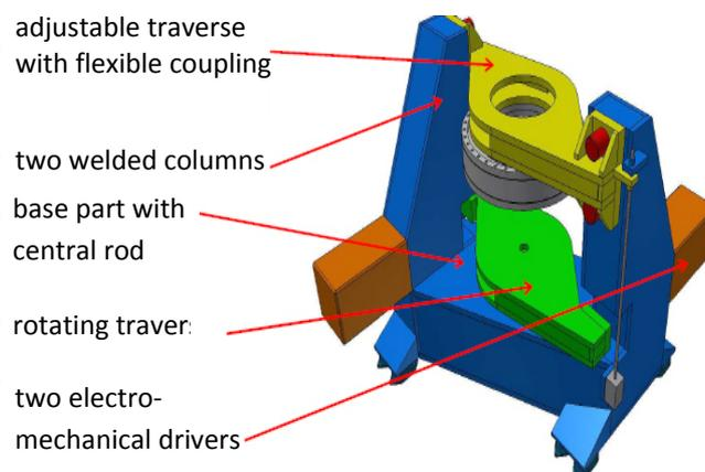
Fig.1: 400 kN·m Torque Calibration Machine with its main parts
