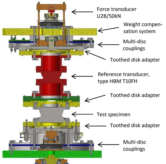
Fig.5: Complete measuring train
