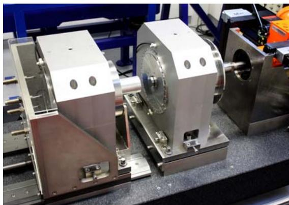
Fig. 1. 250 kN shock force calibration device.
