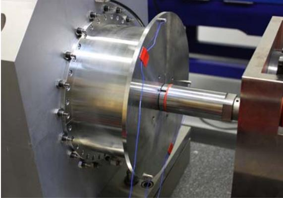
Fig. 4. Mass body M1 applied with additional acceleration sensors.
