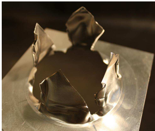
Figure 12. Burst aluminum diaphragm
