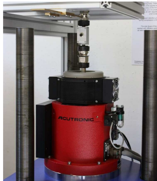
Figure. 13. Dynamic torque measuring device at PTB with the new rotational exciter
