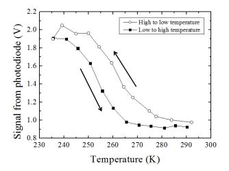
Figure 5. The variation of laser beam power reflected at beamsplitter with temperature change
