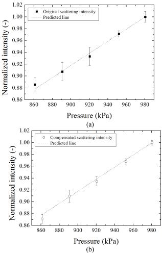
Figure 2. Linearity between pressure variation and (a) original Rayleigh scattering intensity and (b) compensated Rayleigh scattering intensity.
