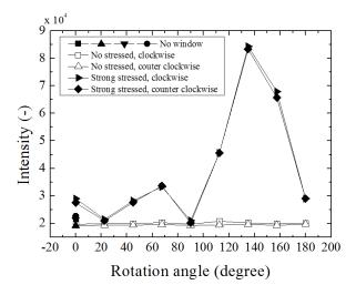
Figure 4. The mechanical stress effect of laser window on scattering intensity
