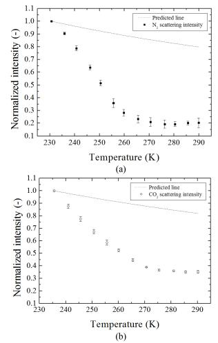
Figure 3. Rayleigh scattering intensity variation with temperature change: (a) nitrogen and (b) carbon dioxide
