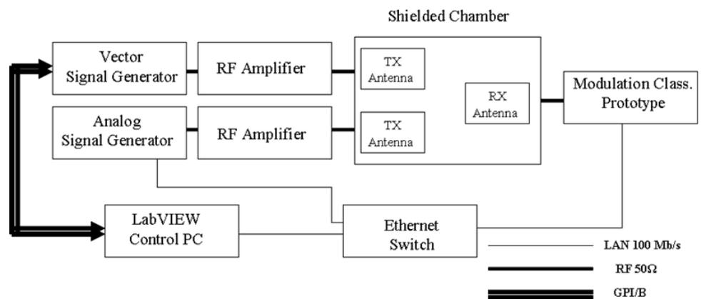
Fig. 3. Test bench setup.
