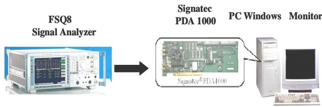
Fig. 2. Modulation Classifier Prototype.
