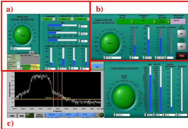
Fig. 4. The VI front panel, divided in three sections: (a) SMIQ03B controls, (b) E8663B controls, (c) FSQ8 and prototype controls.
