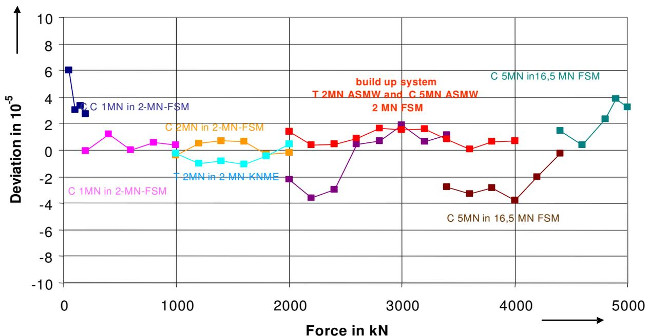
Fig. 3. Results of a comparison between the 5 MN FSM and the 2 MN and 16,5 MN FSM.
