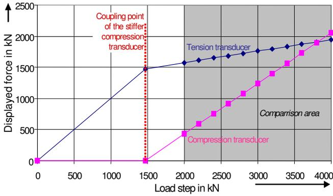
Fig. 2. Characteristics of the two transducers in the build up system.
