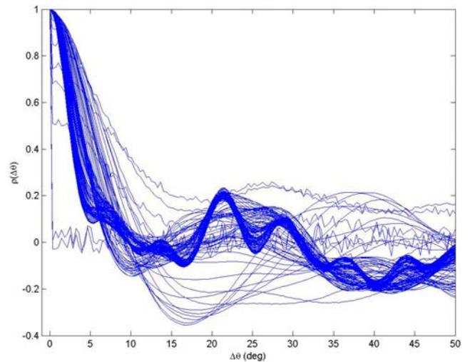
Fig. 3: Evolution of the autocorrelation function of a received pulsed signal inside a reverberation chamber as a function of the angular increment  $\Delta\theta$  of a rotating paddle wheel. Each curve represents a correlation function for a fixed elapsed time  $m\Delta t$  after the start of the pulse  $t_0$  ( $m=0, 1, \dots, 300$ ;  $\Delta t = 5$  ns), taken at different positions of the paddle wheel.
