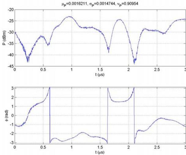
Fig. 6: Close-up of part of measured stir sweep of received power and phase  $\phi$  (use magnification of electronic version to inspect magnitude of ripples).
