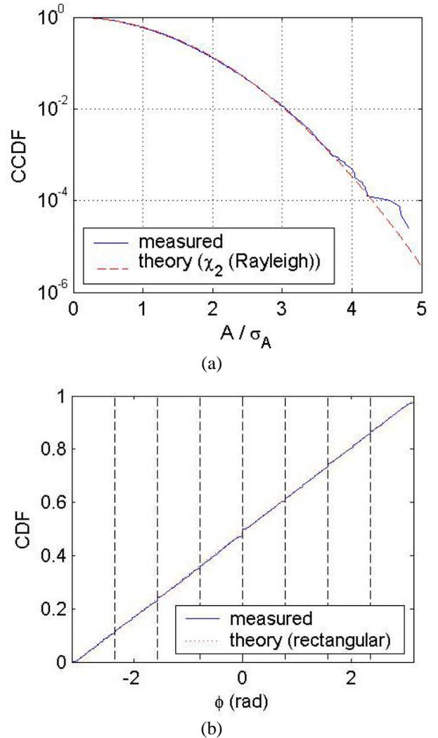
Fig. 5: Measured vs. theoretical probability distributions for mode-stirred operation in “off”-state, at  $t-nt_0=70\mu\text{s}$  ( $n=0, \dots, N-1$ ) for  $N=40,000$  pulse responses across one full paddle wheel rotation; (a) complementary cdf of field magnitude  $A$ ; (b) cdf of phase  $\phi$ .
