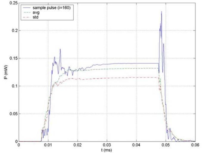
Fig. 2: Typical received distorted signal (blue line) for rectangular input pulse, together with ensemble average (green dashed line) and ensemble standard deviation (red dash-dotted line) for a population of 1000 statistically equivalent multipath environments.
