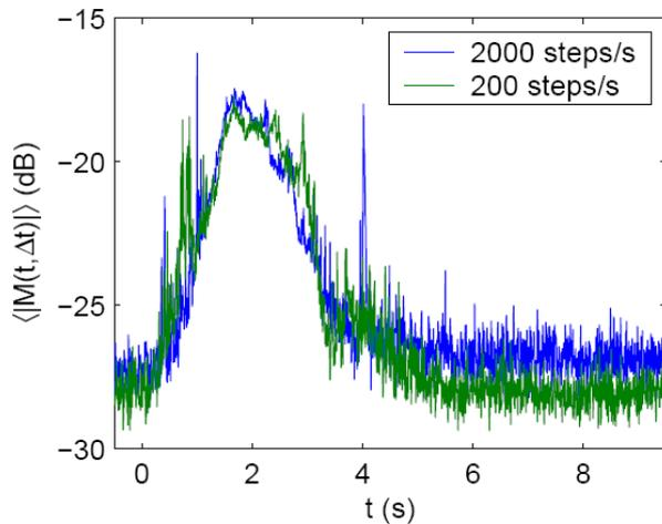
Fig. 1: Ensemble average value of sample modulation index as a function of time during transitions of a moving boundary inside a mode-stirred reverberation chamber.
