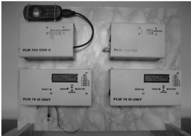
Fig. 4. Designed bus system
