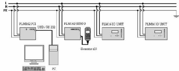
Fig. 2. Structure of the bus system
