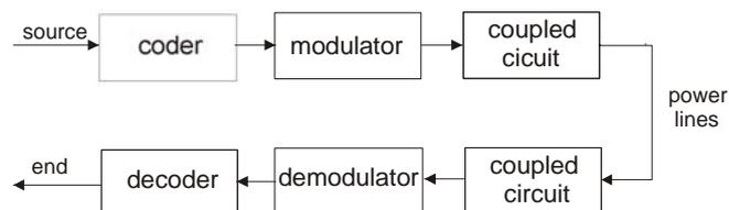
Fig. 1. Setting of the communication parts in the power line system
