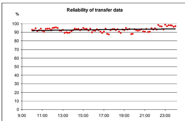
Fig. 6. The reliability of transfer data during a day in a flat, the distance between the transceiver and the receiver 25m
