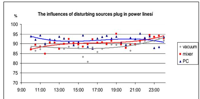
Fig. 7. The influences of disturbing sources in power lines, the distance between the transceiver and the receiver 25m
