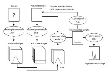
Fig. 2. Block diagram of the super-resolution post-processing
