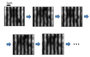
Fig. 17. Examples of modulated scattered light images by standing wave illumination shift (incident light directions are right & left)
