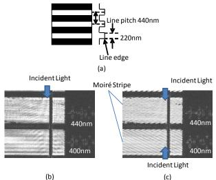
Fig. 14. (a) Schematic diagram of an L&S pattern(b) Observed image of an L&S pattern (one incident light)(c) Observed images (incident light directions are up & down)
