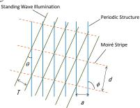
Fig. 13. The schematic diagram of moiré stripe
