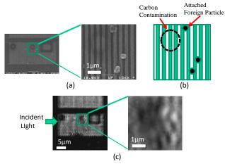
Fig. 16. Images of the sample (a) obtained by SEM (b) The schematic diagram (c) obtained by the equipment
