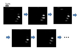
Fig. 18. Examples of modulated scattered light images by standing wave illumination shift (incident light directions are up & down)
