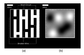
Fig. 8. (a) Short circuit and broken wires on line & space pattern (b) Normal imaging of *NA*0.95
