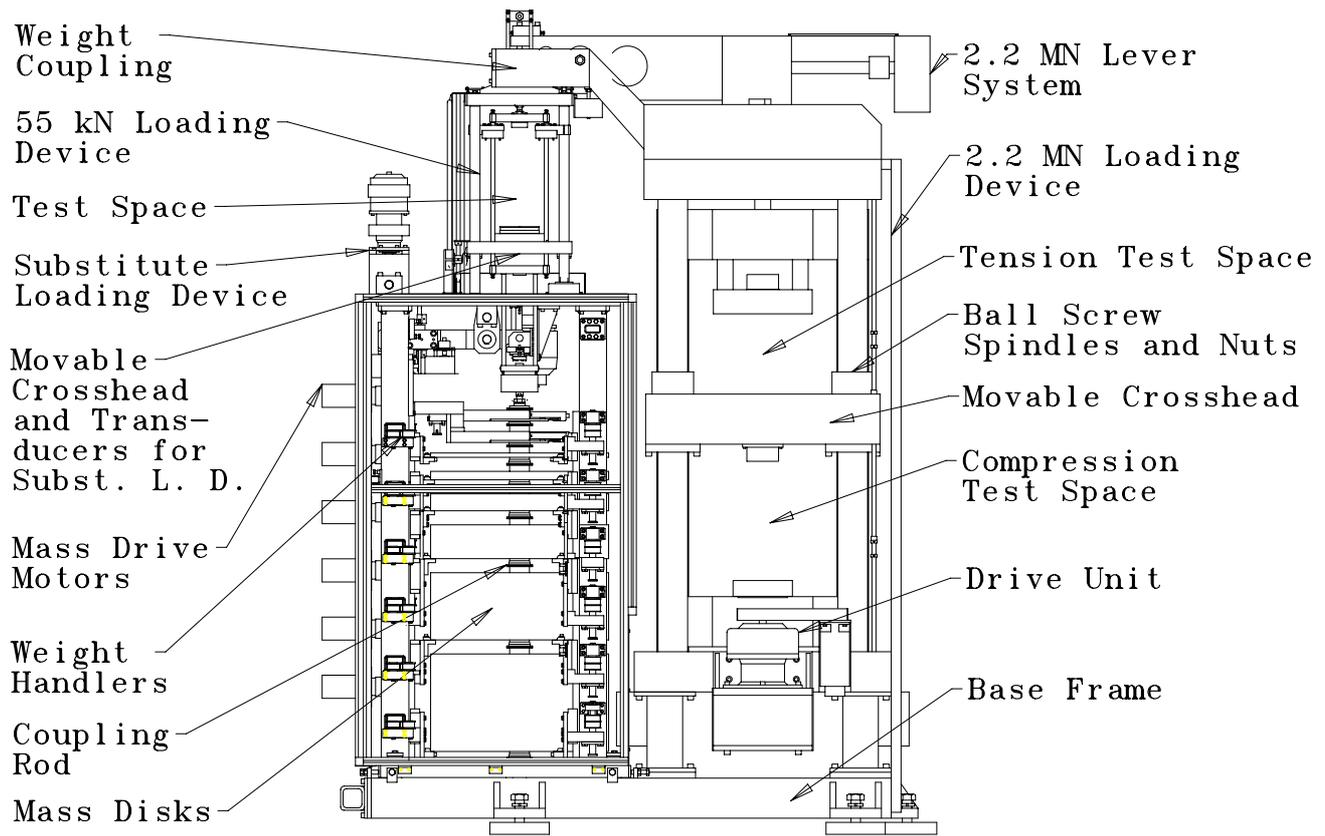
Fig. 1. General assembly drawing of machine with main components
