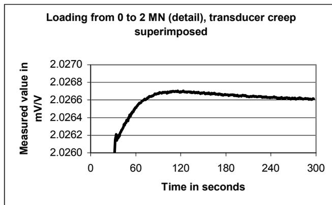
Fig. 5b. Typical load stability (lever machine)
