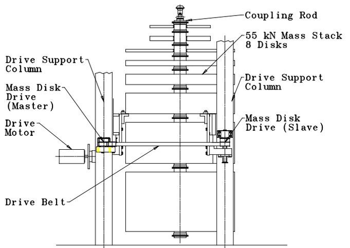
Fig. 3. Mass stack section
