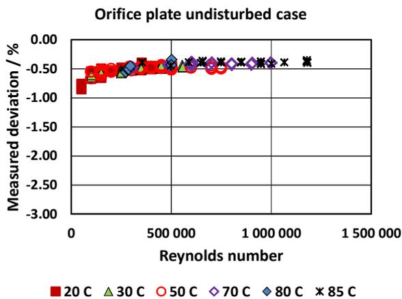
Figure 3. Results of undisturbed measurements: Measurement deviation of the orifice plate in dependence of Reynolds number at different temperatures.
