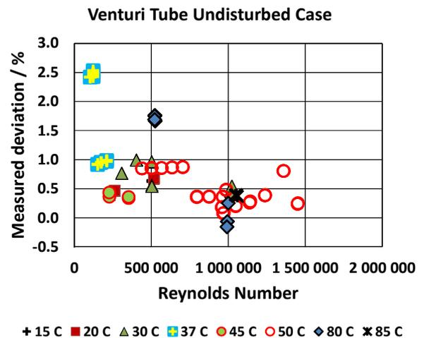
Figure 5. Results of undisturbed measurements: Measurement deviation of the Venturi in dependence of Reynolds number at different temperatures.
