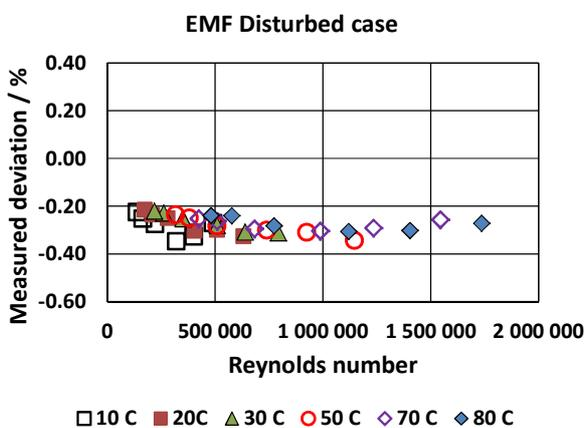
Figure 8. Results of disturbed measurements: Measurement deviation of the EMF in dependence of Reynolds number at different temperatures.
