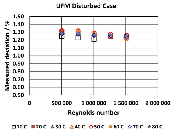
Figure 2. Results of disturbed measurements: Measurement deviation of the UFM in dependence of Reynolds number at different temperatures.
