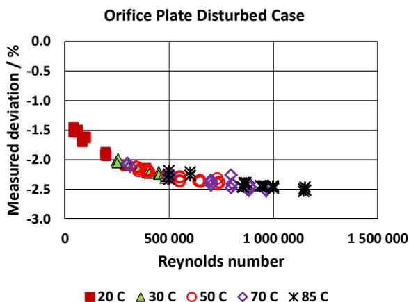
Figure 4. Results of disturbed measurements: Measurement deviation of the orifice plate in dependence of Reynolds number at different temperatures.
