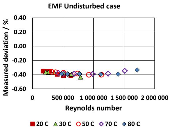
Figure 7. Results of undisturbed measurements: Measurement deviation of the EMF in dependence of Reynolds number at different temperatures.
