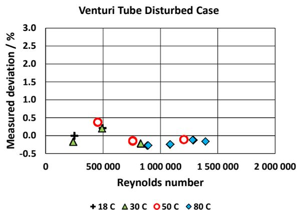
Figure 6. Results of disturbed measurements: Measurement deviation of the Venturi tube in dependence of Reynolds number at different temperatures.
