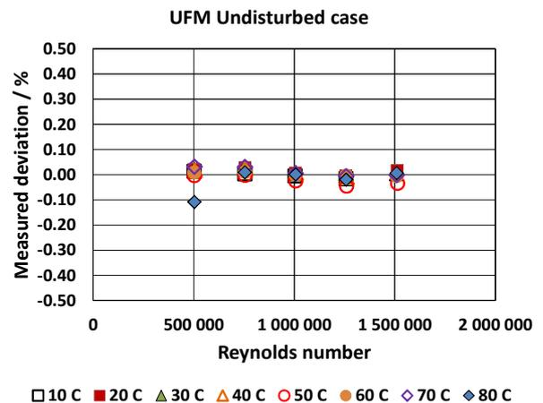
Figure 1. Results of undisturbed measurements: Measurement deviation of the UFM in dependence of Reynolds number at different temperatures.
