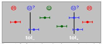
Figure 1: Conforming (green) and non-conforming (red) measurands. The blue points are not conforming and not non-conforming.
