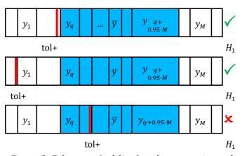
Figure 5: Tolerances (red lines) and coverage intervals around  $\bar{y}$  (blue cells) while testing the alternative hypothesis  $H_1$ . In the upper and middle rows the coverage interval is within tolerance and  $H_1$  is accepted. In the lower row the lower tolerance is in the coverage interval and  $H_1$  is rejected.
