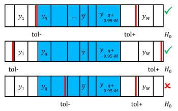
Figure 4: Tolerances (red lines) and coverage intervals around  $\bar{y}$  (blue cells) while testing the null hypothesis  $H_0$ . In the upper and middle rows the coverage interval is within tolerance and  $H_0$  is accepted. In the lower row the lower tolerance is in the coverage interval and  $H_0$  is rejected.
