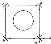
Fig.1. Schematic view of Sagnac experiment. Light from S is split in two parts: the first follows the path ABCDAO in the same direction of rotation, the second ADCBAO in the opposite direction, they interfere in O.
