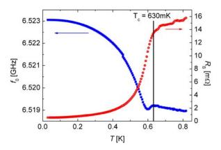
Fig. 3. Temperature dependence of stripline resonator frequency  $f_0$  and sample surface resistance  $R_s$  measured on a CeCu<sub>2</sub>Si<sub>2</sub> single crystal sample.
