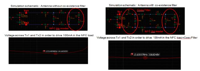
Figure 11: Simulation of the NFC antenna with and without the co-existence filter
