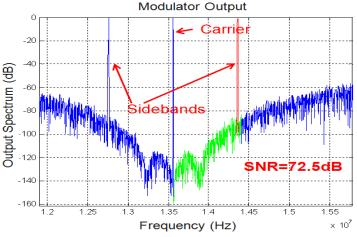
Figure 9: 4-bit modulator output spectrum with 100% ASK signal
