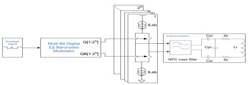
Figure 7: Block diagram of proposed multi-bit transmitter architecture
