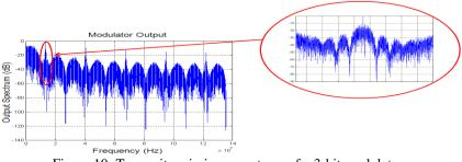
Figure 10: Transmit emissions spectrum of a 3-bit modulator
