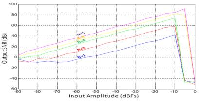
Figure 8: SNR versus Input Amplitude Sweeps for different number of bits in the quantizer
