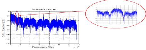
Figure 6: Transmit emissions for a mono-bit modulator
