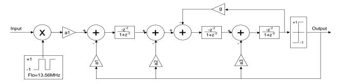
Figure 4: Block diagram of the band-pass modulator
