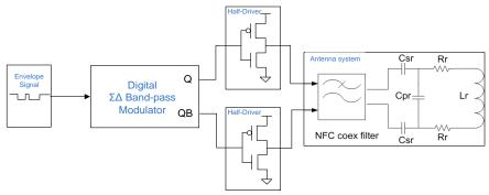
Figure 3: Block diagram of proposed single-bit transmitter architecture
