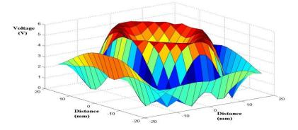
Figure 2: A graph of voltages seen in the field of the NFC enabled device.
