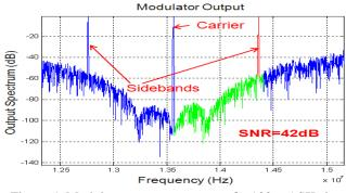
Figure 5: Modulator output spectrum of a 100% ASK signal
