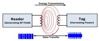
Figure 1: Block diagram illustrating a basic NFC system
