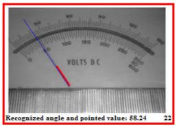
Figure 6. Result for analogue meter. Recognized angle=58.24° and meter indication=22 volts.
