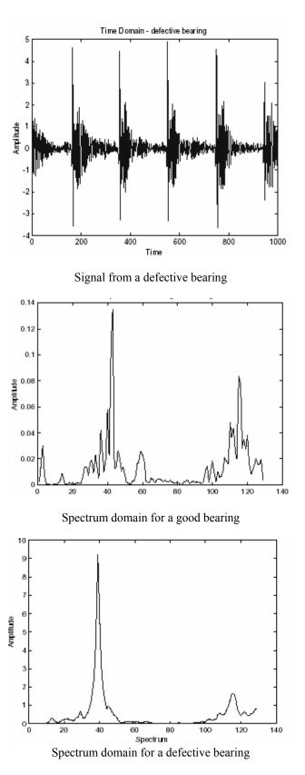
Figure 8 Signals and spectrum domain from a normal and a defective bearing
