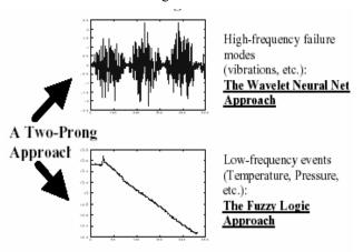
Figure 1 The two-prong approach of the diagnostic module
