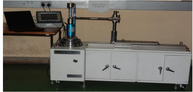
Fig. 8: Automatic Torque Wrench Calibrator used at KEBS.
