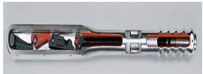
Fig. 4: Multi-lever inside mechanism of a click torque wrench [9].
