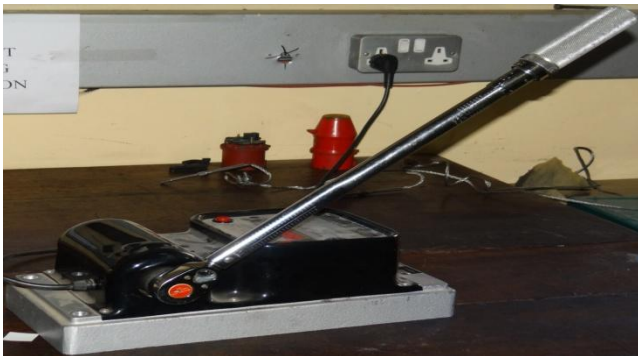
Fig.7: Manual calibration device (digital meter) used at KEBS
