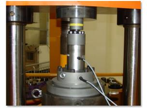
Fig. 5: The figure shows the build-up system mounted in the 1MN force standard machine (fsm) of PTB.
