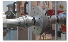
Fig. 2: The figure shows the build-up system mounted in the  $1kN\cdot m$  torque standard machine of PTB.
